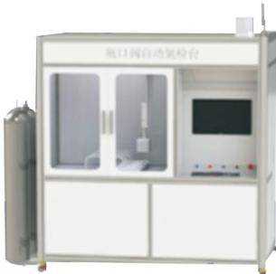
Function: Test the sealing ability of parts such as the car-mounted hydrogen bottle bottle valve
