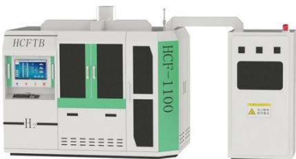
Function: Test the performance of the components in the hydrogen low pressure section of the fuel cell
