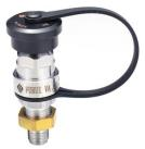
The hydrogen port is a specially designed hydrogen filling seat for fuel cell vehicles; the flow chann el is smooth and noiseless; the built-in filter element filters dust particles and provides sealing performance; the interface size is designed according to GB/T26779 standard, with more precise size control and better cooperation with the hydrogen filling gun; it is qualified by the special inspection institute for 30,000 times life test, reducing product maintenance and downtime.
